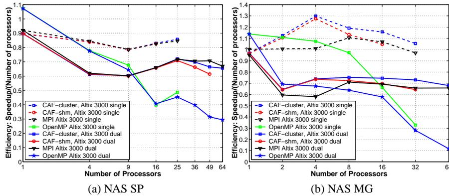
**Fig. 8.** Comparison of parallel efficiencies for NAS SP and NAS MG for MPI, CAF with general communication and CAF with shared memory communication, as well as OpenMP versions on an SGI Altix 3000.
