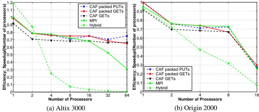
**Fig. 7.** Comparison of parallel efficiencies (per iteration) for Spark98 (sf2 trace) for CAF, MPI and hybrid versions on an SGI Altix 3000 and an SGI Origin 2000.
